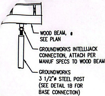
1A.A: FLAT PLATE W/ WOOD BEAM
