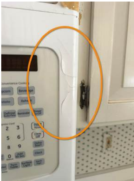
Area of microwave main housing is damaged/cracked
