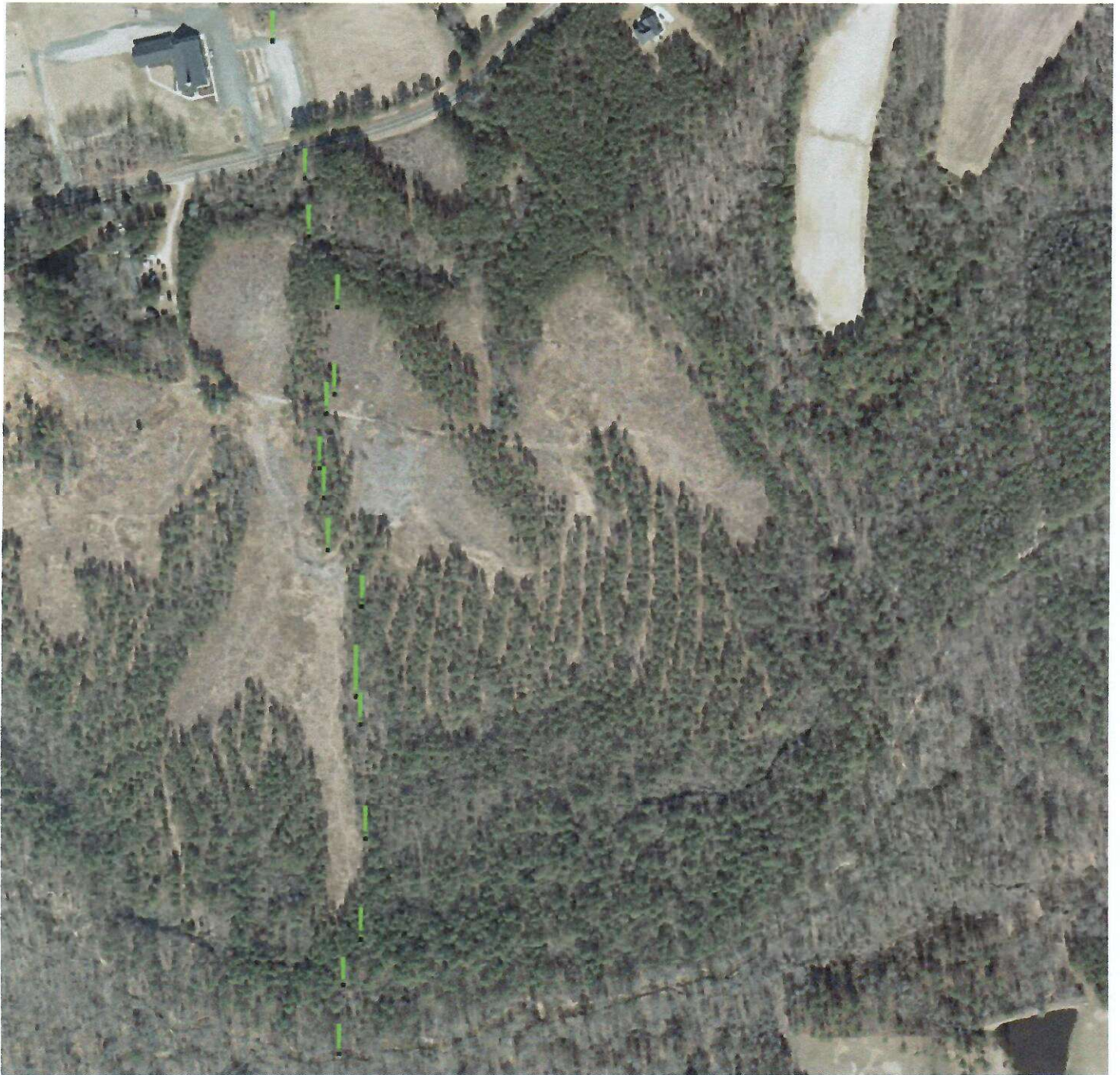
Figure 7. Locations of magnetic highs along the dike from Walters Road south to the big creek. Locations are at the base of each mark; locations of the two wells are also shown. They are flagged in the field. The Appendix contains GPS coordinates. The dike strikes approximately 355^{\circ} and dips west at about 85^{\circ} .
