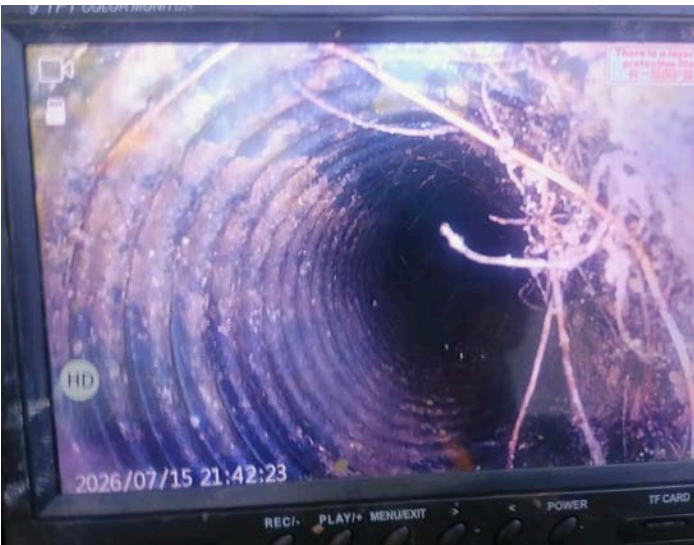
Minor sludge are roots in the leach field lines
