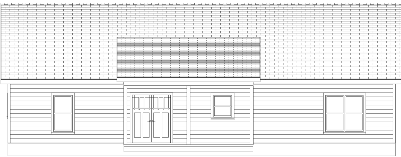
E3 EXTERIOR ELEVATION BACK 1/8 IN = 1 FT
