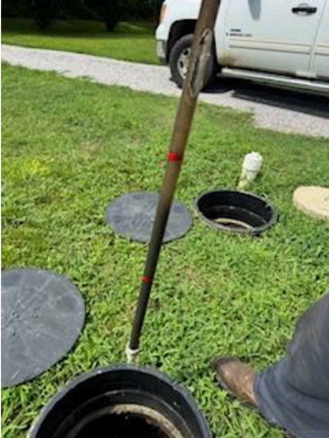
TANK LAYOUT – Sludge judge on INLET
